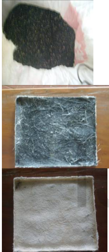
PLATE 4: Recycled Plastic Resin and Casting Progress of GFRP Laminates
